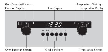
The oven power indicator illuminates as long as the oven is in operation.
